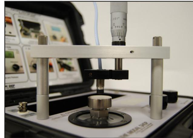
Eddy current proximity probe static and dynamic output checked with the 9100-PPA01 fixture
